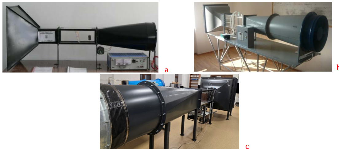
FIG. 7 Wind tunnel, a Tunell custom (WT1), b Tunell SES 115 (WT2), c Tunell ELECO (WT3)
