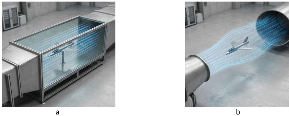
FIG.2 Typology of experimental chambers of open-flow subsonic wind tunnels, a. closed chamber , b. open chamber
