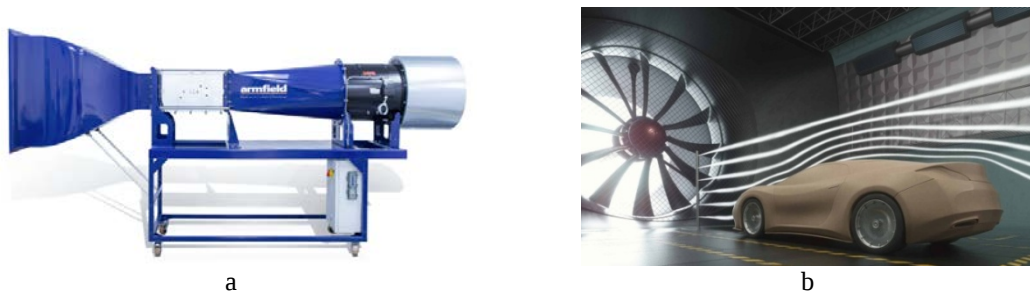
FIG. 3 Experimental chamber typology a.for reduced scale model [7], for real model [8]
